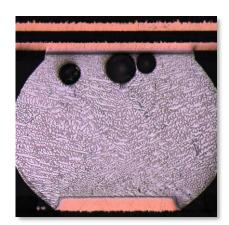
Our cross-section services include a detailed analysis report of samples in PDF, carried out by one of our experts, where the identified problems and non-conformities of the assemblies are specified, dimensions are detailed on each image, such as intermetallic union or voids in the solder or other defects detected in assembly.
